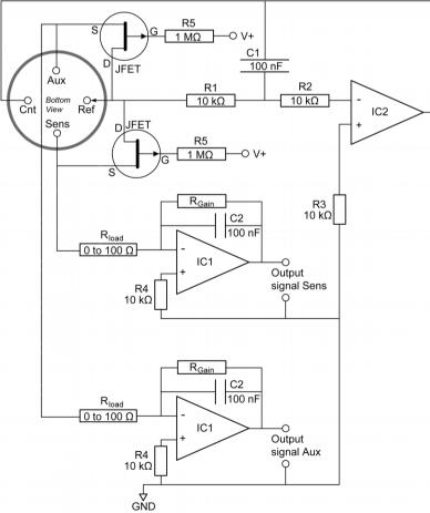
Figure 1 Schematic diagram of the electronic circuit for 4-electrode-sensor
